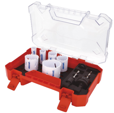
Item No. 101747B 9PCS PLUMBERS' KIT in plastic case (6) Bi-metal hole saws: 19, 22, 29, 38, 44, 57mm (3/4", 7/8", 1-1/8", 1-1/2", 1-3/4", 2-1/4"); (1) 3/8" hex shank arbor with pilot bit; (1) 7/16" hex shank arbor with pilot bit; (1) arbor adapter.
