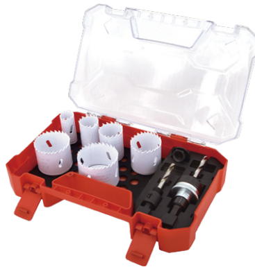
Item No. 101746B 9PCS ELECTRICIANS' KIT in plastic case (6) Bi-metal hole saws: 22, 29, 35, 44, 51, 64mm (7/8", 1-1/8", 1-3/8", 1-3/4", 2", 2-1/2"); (1) 3/8" hex shank arbor with pilot bit; (1) 7/16" hex shank arbor with zinc-plated knurled locking collar and pilot bit; (1) arbor adapter.
