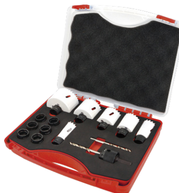
Item No. 110601B 14PCS QUICK CHANGE BI-METAL HOLE SAW KIT in plastic case (6) Bi-metal hole saw with adapter nut: 22, 29, 35, 44, 51, 64mm (7/8", 1-1/8", 1-3/8", 1-3/4", 2", 2-1/2"); (1) 7/16" hex shank quick change arbor with pilot bit; (1) replacement pilot drill; (2) adapter nut with 1/2"-20UNF thread; (4) adapter nut with 5/8"-18UNF thread.
