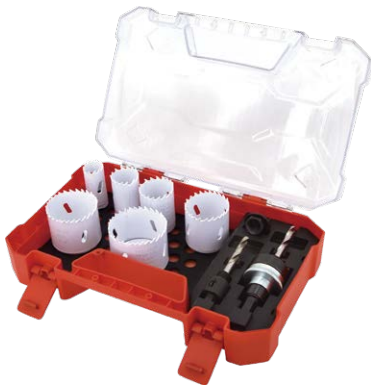
Item No.101748 9PCS PLUMBERS' KIT in plastic case (6) Bi-metal hole saws:19,22,29,38,44,57mm (3/4", 7/8", 1-1/8", 1-1/2", 1-3/4", 2-1/4"); (1)3/8" hex shank arbor with pilot bit; (1)7/16" hex shank arbor with zinc-plated knurled locking collar and pilot bit; (1)arbor adapter.
